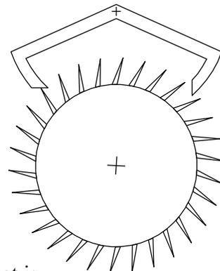
The escapement wheel is coupled to a gear chain that is powered by a mainspring or a weight. The gear chain also turns the hands of the clock. If the rocker arm is removed, the escapement wheel—and the clock’s hands—would spin rapidly until the power source was exhausted. The escapement lets a small, metered parcel of energy that is stored in the mainspring or weight to *escape*.
