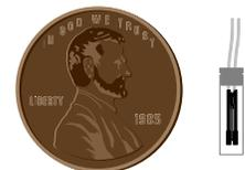
oscillate at its natural frequency of 32,768 Hz. This frequency is 2 to the power of 15. By dividing the frequency in half repeatedly 15 times, the final frequency will be 1 Hz. or 1 pulse every second. This 1 Hz. signal can drive a stepping motor that moves the second hand of an analog watch or drive the seconds digit counters of a digital watch. Shown below is a chain of 15 “flip-flops.”
